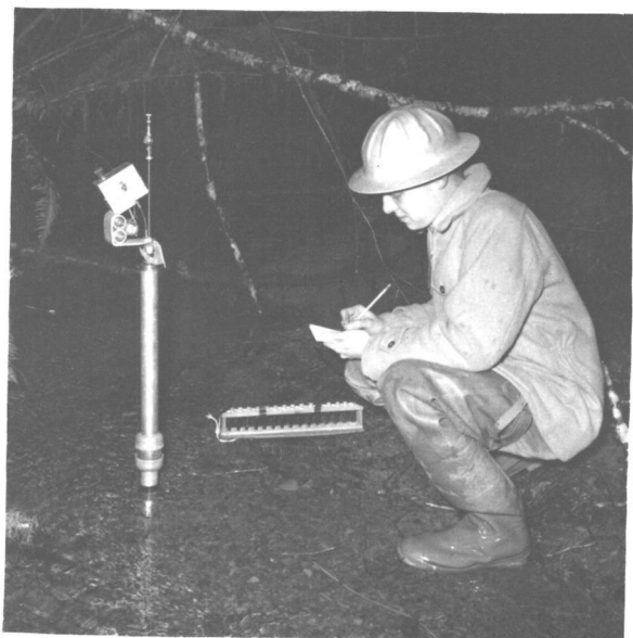
Figure 8. Obtaining readings of apparent velocity of ground water.
